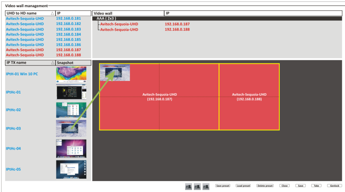
Figure 5-23 Drag the TX Snapshot to the Blank Window in the 2x2 Wall Template
