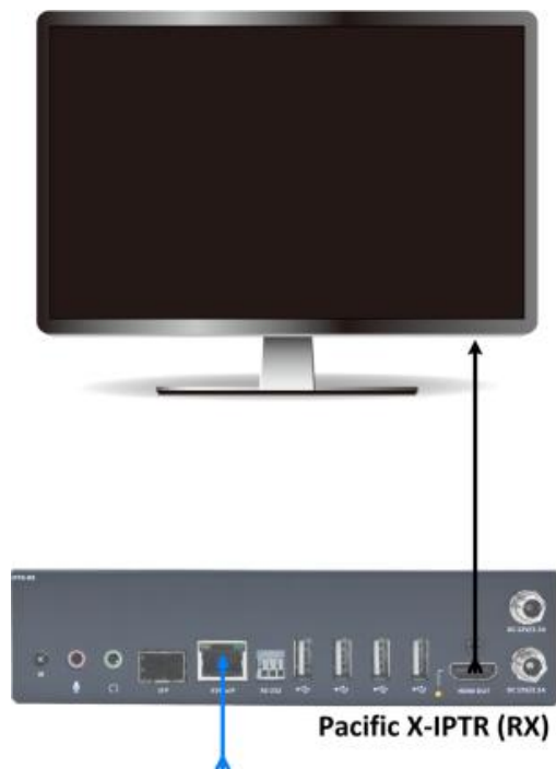
Figure 2-12 Connections to the Pacific X-IPTR (RX) Diagram
