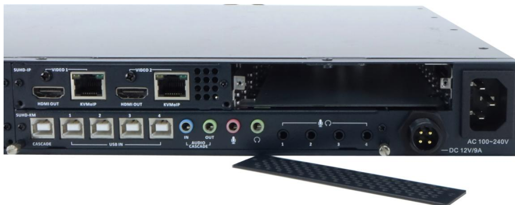
Figure 2-2 Remove the Back Plate
