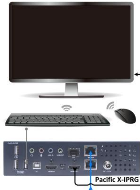
Figure 2-13 Connections to the Pacific X-IPRG Diagram
