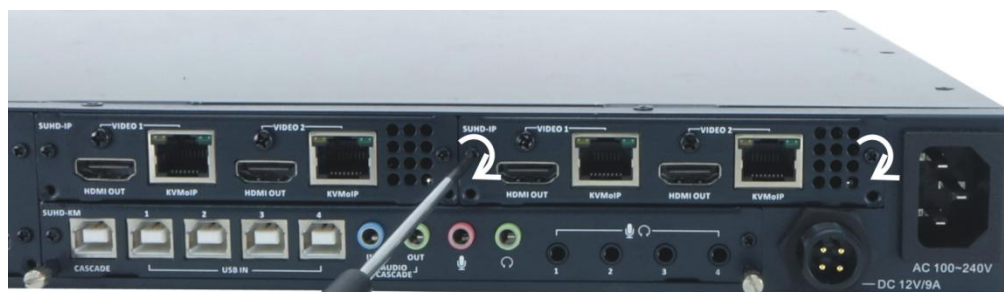
Figure 2-4 Tighten the Module Screws on Both Sides
