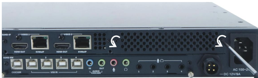
Figure 2-1 Remove the Two Plate Screws
